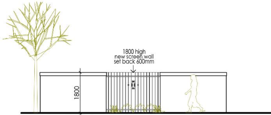
elevation of wall with palisade panel
