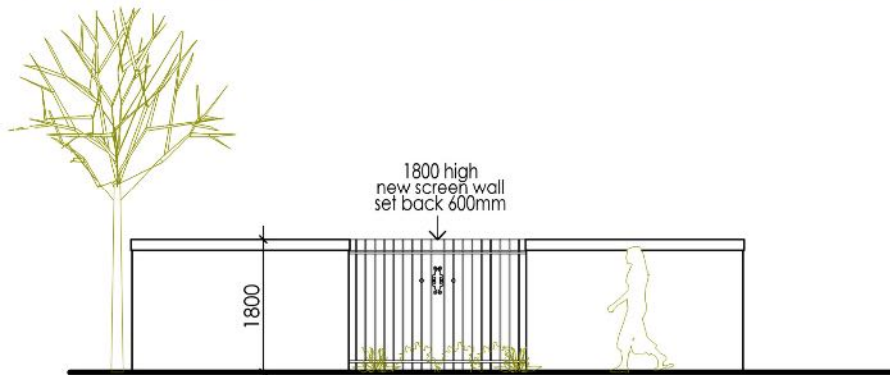
elevation of wall with palisade panel
